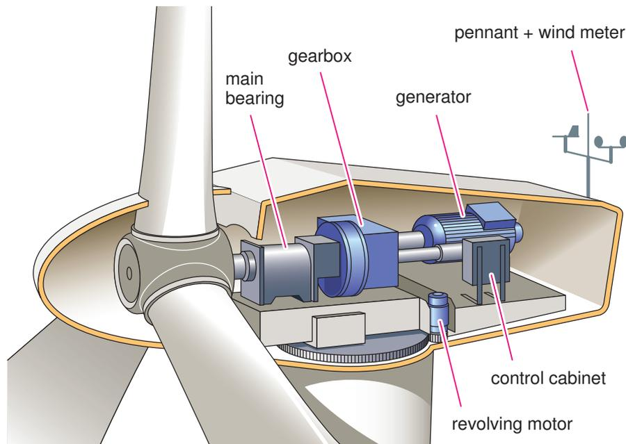
Figure 5: Cross-section of a wind turbine nacelle
