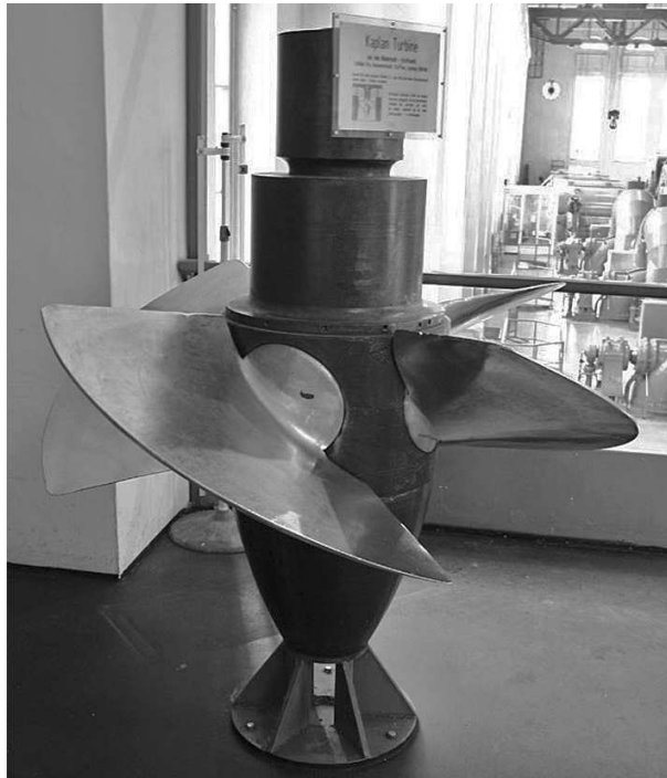
Figure 12: Water turbine propeller
